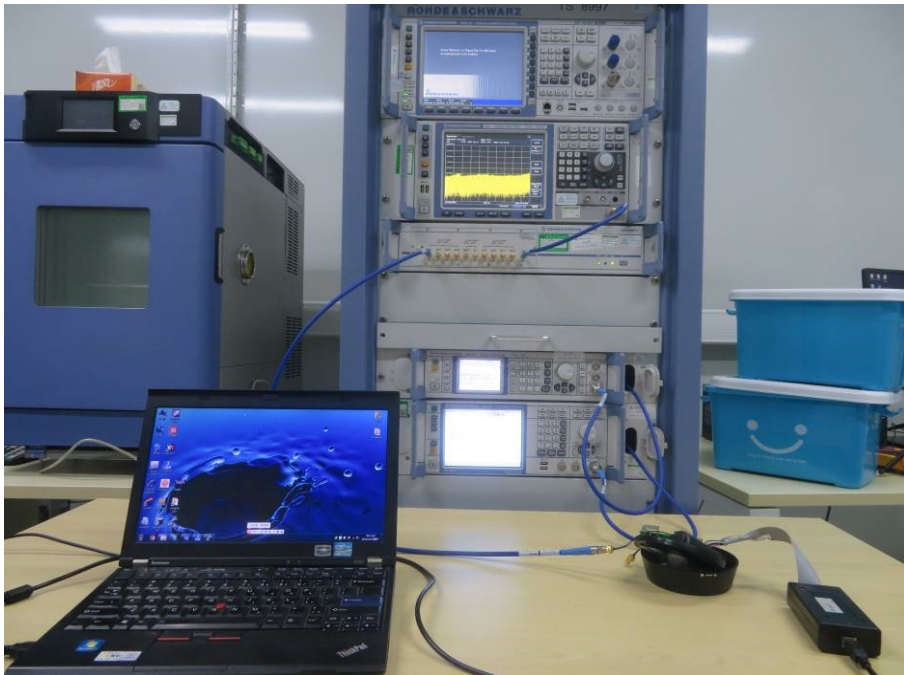
Photograph 1: Set-up for Radio Spectrum Test
