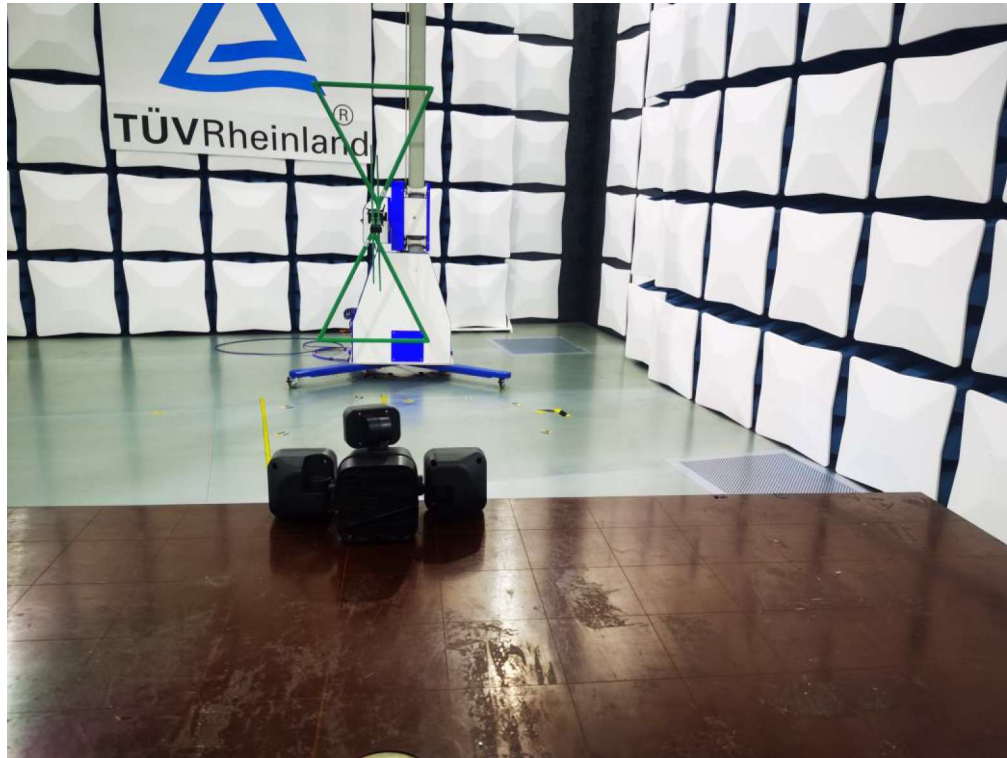
Photograph 2: Set-up for Radiated Emission, above 1GHz
