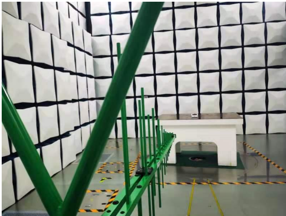
Photograph 2: Set-up for Radiated Emission, above 1GHz
