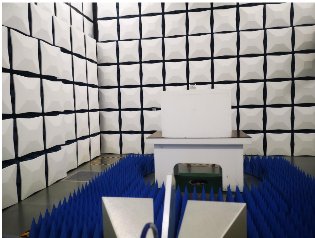
Photograph 2: Set-up for Radiated Emission, above 1GHz
