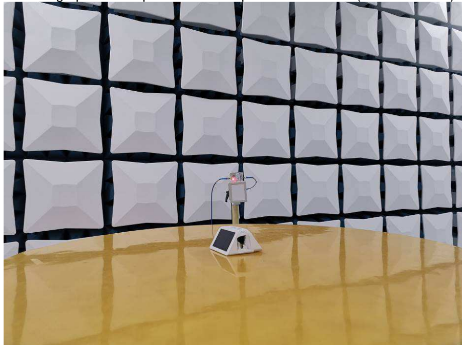
Photograph 2: Set-up for Radiated Spurious Emissions (18GHz-25GHz)
