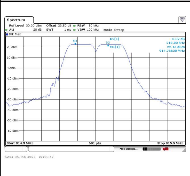
Channel Separation Plot on Channel 64 - 65
