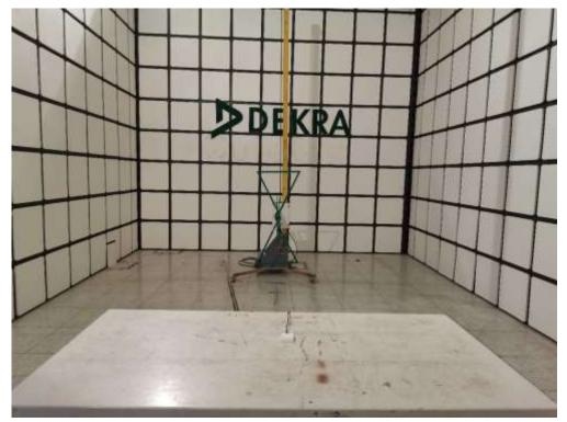
Description: Radiated Emission Test Setup for 1~18GHz
