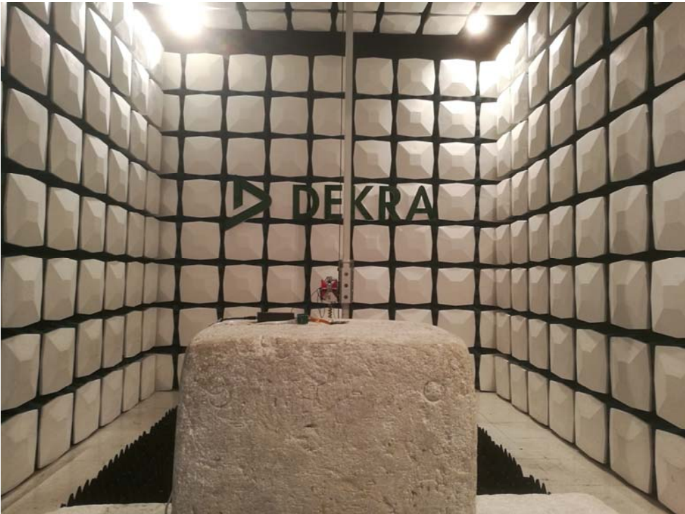
Description: Radiated Emission Test Setup for 1~18GHz
