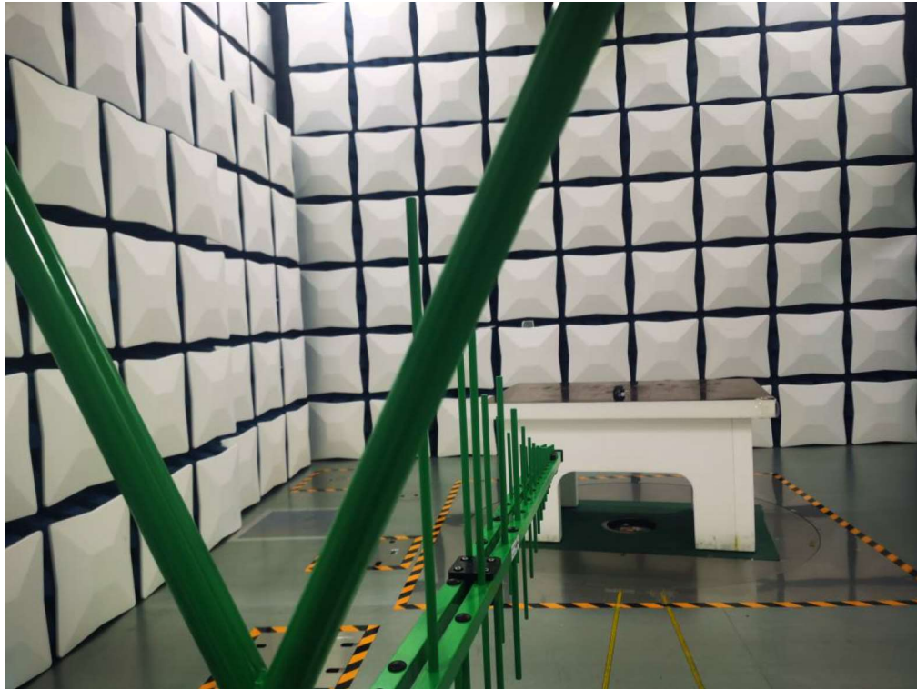
Photograph 2: Set-up for Radiated Emission, above 1GHz
