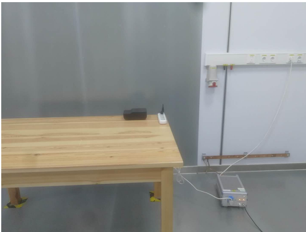
Fig. 4 Power line conducted emission setup photo
