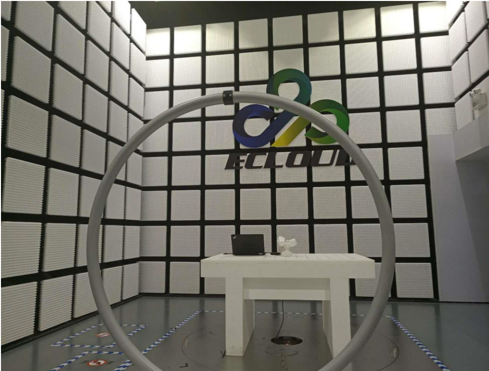
Fig. 1 Radiated emission setup photo(Below 30MHz)
