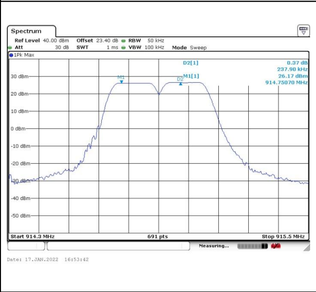
Channel Separation Plot on Channel 64 - 65
