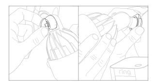
Do not remove your Floodlight Cam from the ball socket on the base.
