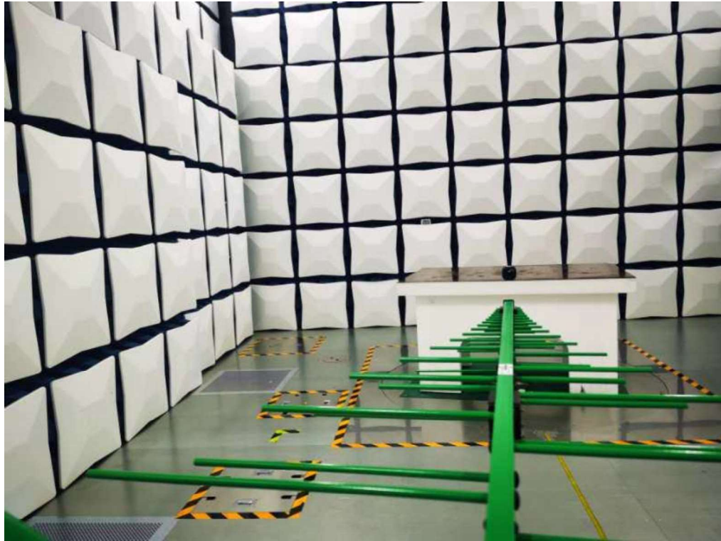
Photograph 2: Set-up for Radiated Emission, above 1GHz
