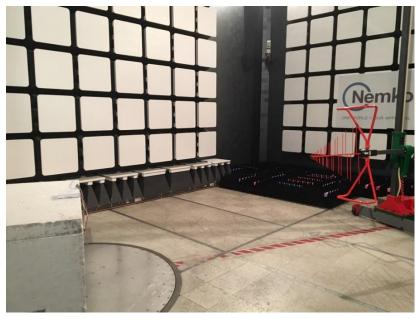
Figure 1.1-2: Radiated emissions setup photo – below 1 GHz
