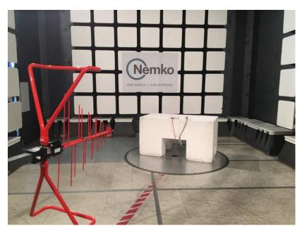
Figure 1.1-1: Radiated emissions setup photo – below 1 GHz
