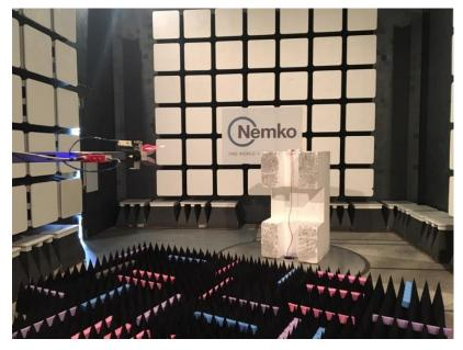
Figure 1.1-4: Radiated emissions setup photo – above 1 GHz
