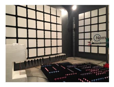
Figure 1.1-3: Radiated emissions setup photo – above 1 GHz
