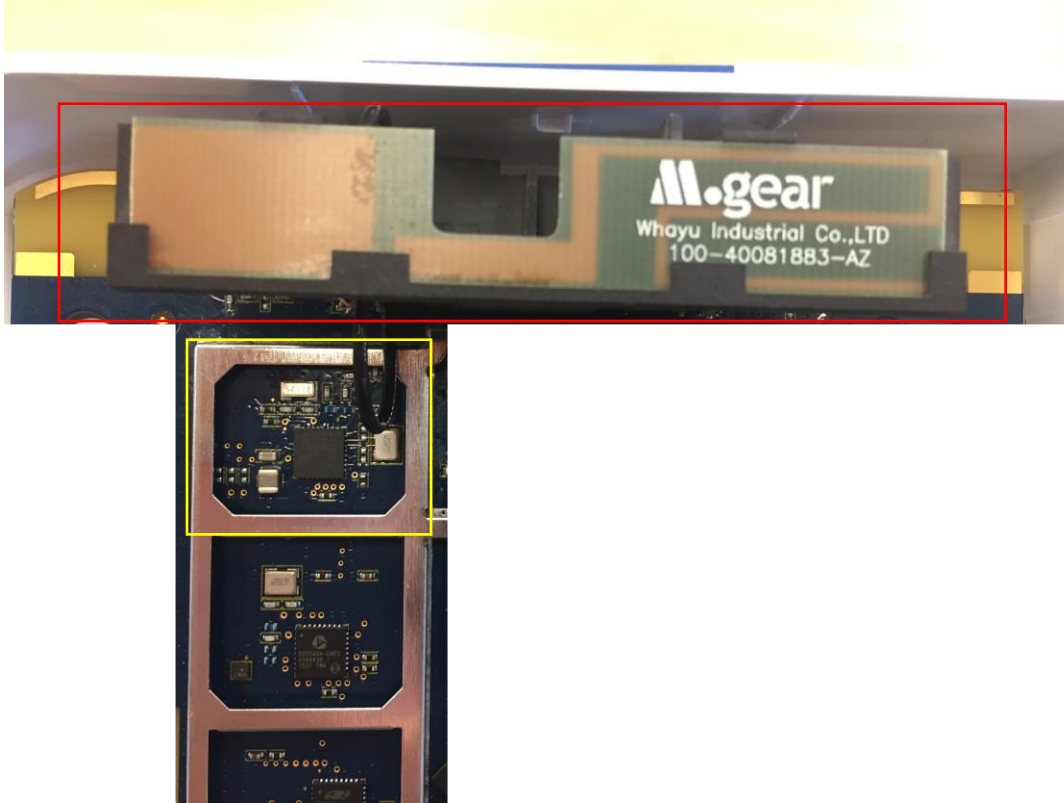
T11310 Radio – antenna in red, radio in yellow
