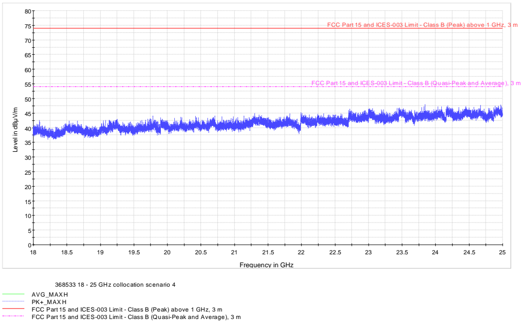
Figure 8.1-26: Radiated spurious emissions products from co-located transmitters within 18 - 25 GHz, Configuration 4
