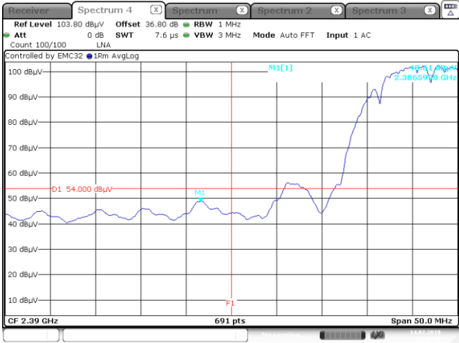
Figure 8.7-2: Unwanted emissions in restricted band Average 2390 MHz 802.11b, low channel
