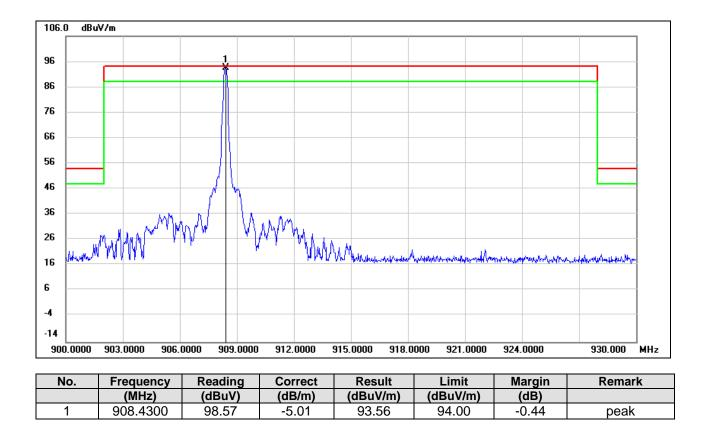
Note: 1. Measurement = Reading Level + Correct Factor. 2. QP detector.
