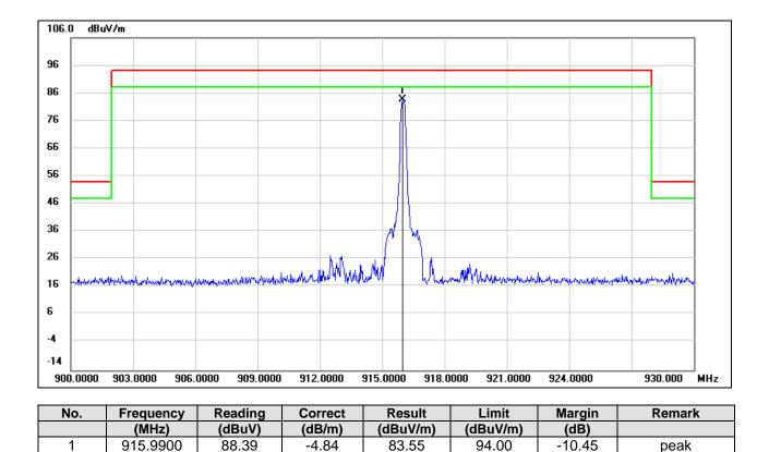
Note: 1. Measurement = Reading Level + Correct Factor.
