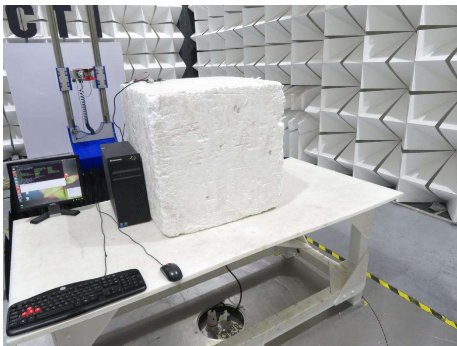
Radiated spurious emission Test Setup-3(Above 1GHz)
