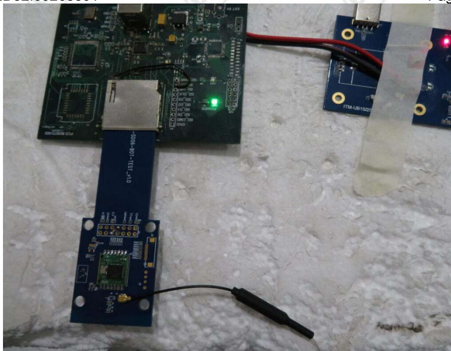
Radiated spurious emission Test Setup for close-up
