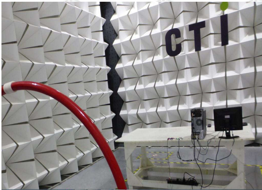
Radiated spurious emission Test Setup-1(Below 30MHz)
