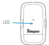
Sensor is switched on with the magnet switch tool by holding it against the sensor's magnetic switch.
