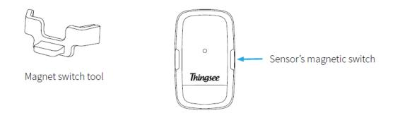
Hold the magnet switch tool against the sensor (see the pic) until the LED indicator starts to blink brightly for one minute.
