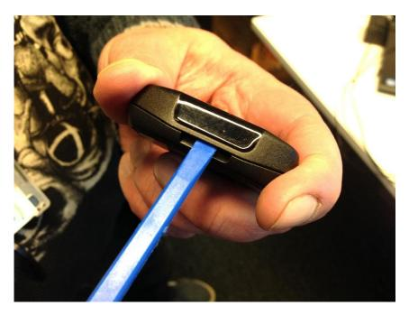
If the device is already attached to some surface, opening needs to be performed with a special tool:
