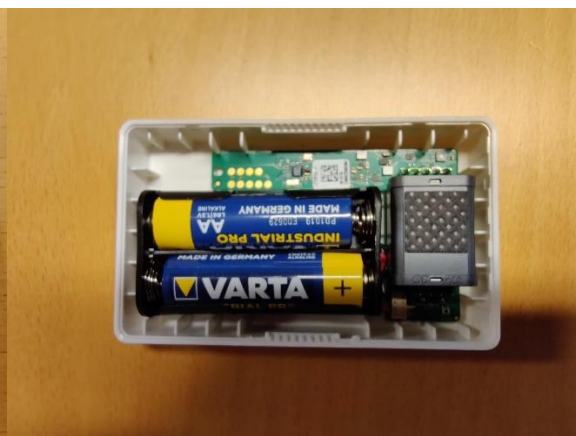
4 A cover inside with PWB and batteries
