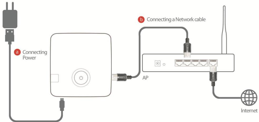
Connect the network cable and the USB power cable in the package as shown in the picture above.
