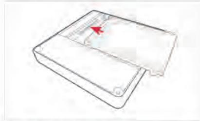
③ Put the hard disk in the SATA connector port. Then, align the hard disk to the holes in the body.
