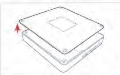
② Lift the back cover of the AIRDisk. Beware that one side that is attached to main body.
