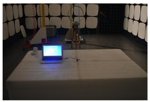
3. Radiated emission (9KHz-30MHz)
