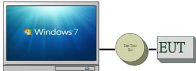
Fig. 2-1 Radiated & Conducted (Antenna Port) Emission Configuration
