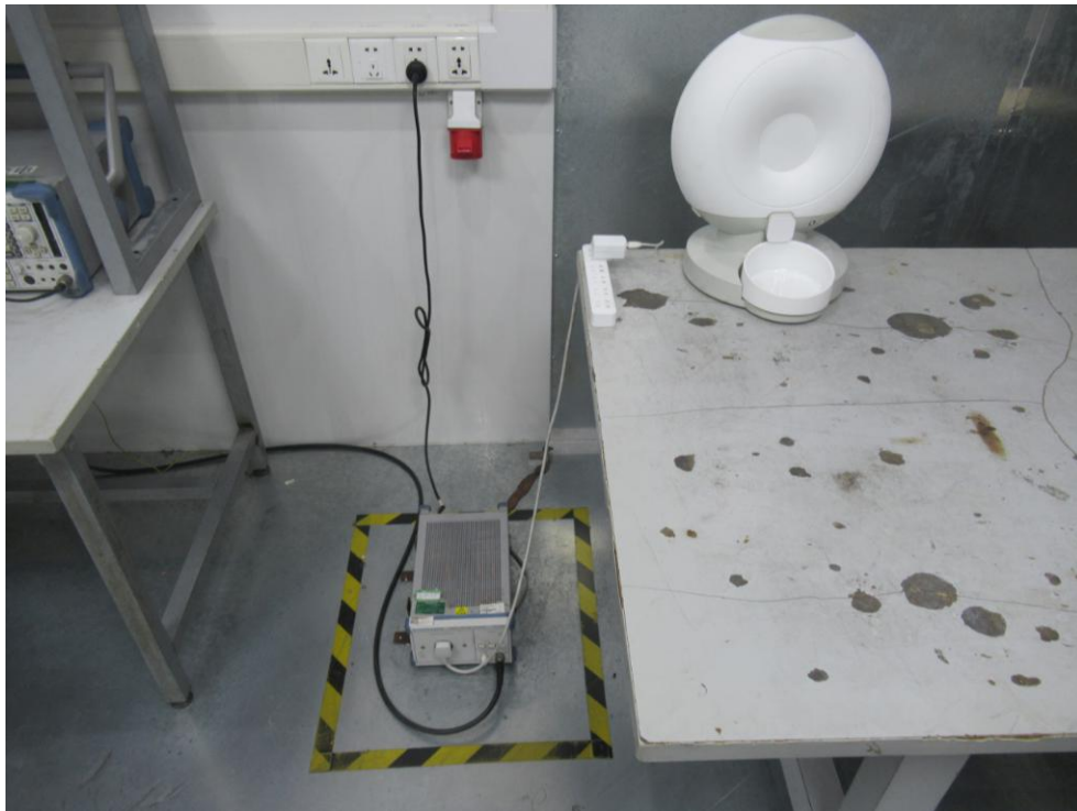
FCC ID: 2AETS-PPCPF01 Photo of Conducted Emission Measurement
