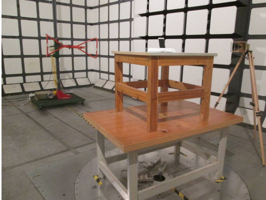
Radiated Emissions Test View (Below 1 GHz)
