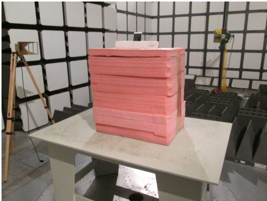
Radiated Emissions Test View (Above 1 GHz)
