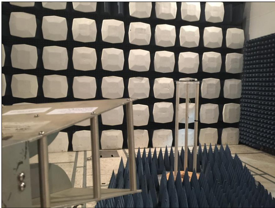
Photograph 2. Radiated Spurious Emissions, Above 1GHz, Test Setup
