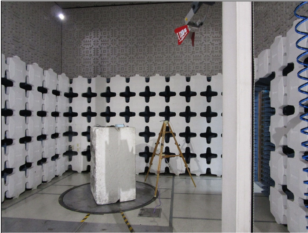
Test Setup for Radiated Spurious Emissions – Above 1GHz Horizontal Antenna Polarization
