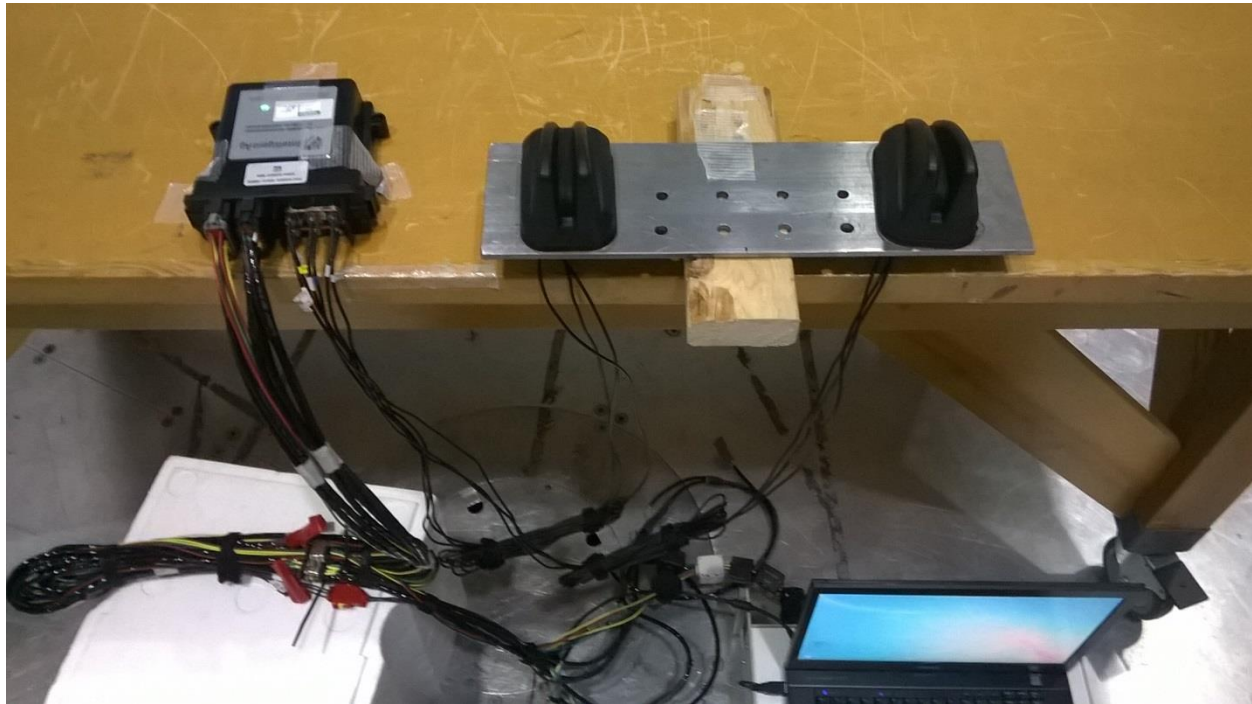
Figure 2 - Radiated emissions, 30MHz - 1GHz
