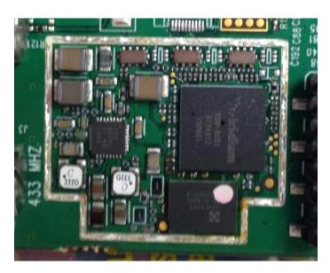
Figure 7 - Satellite communication radio, upper portion, shield removed
