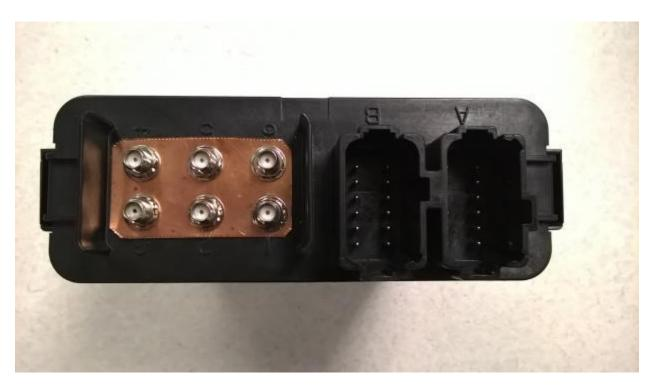
The baseplate will be nickel plating over phosphor bronze for production. On production units, the plate will appear more silver from the nickel plating.
