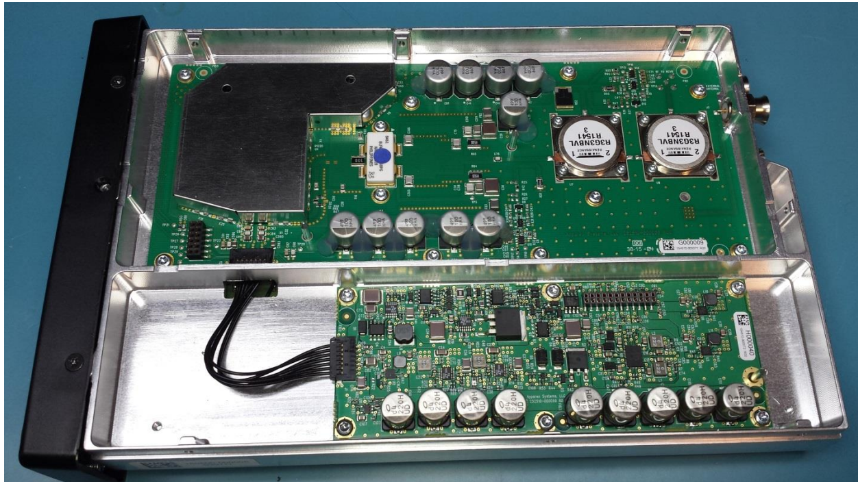
Figure 5 - Power and Transmit cavity with TX board shield on
