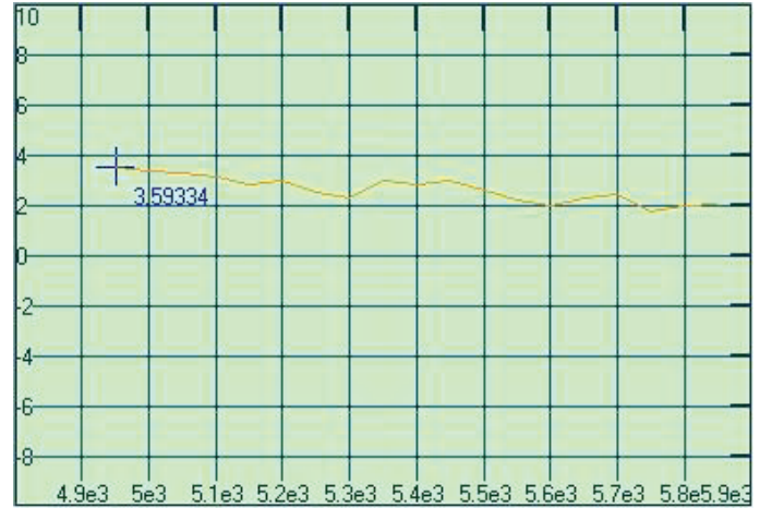
Maximum Peak Gain at 4950 MHz : 3.59 dBi
