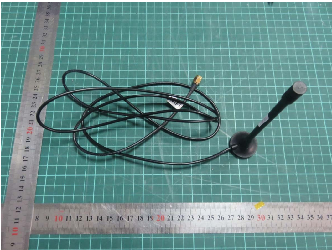
c: Wi-Fi antenna
