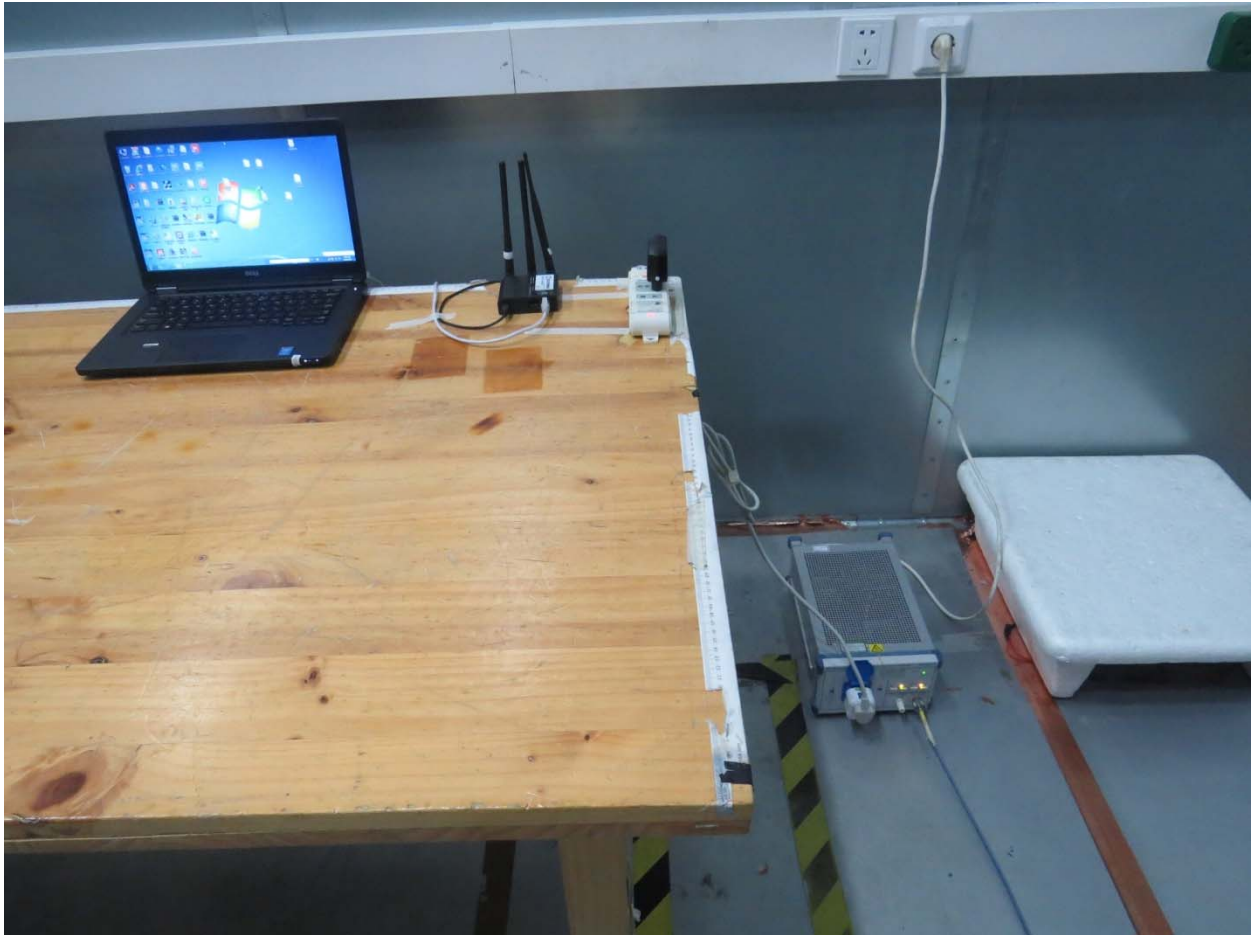
Picture 3 Conducted Emission Test Setup
