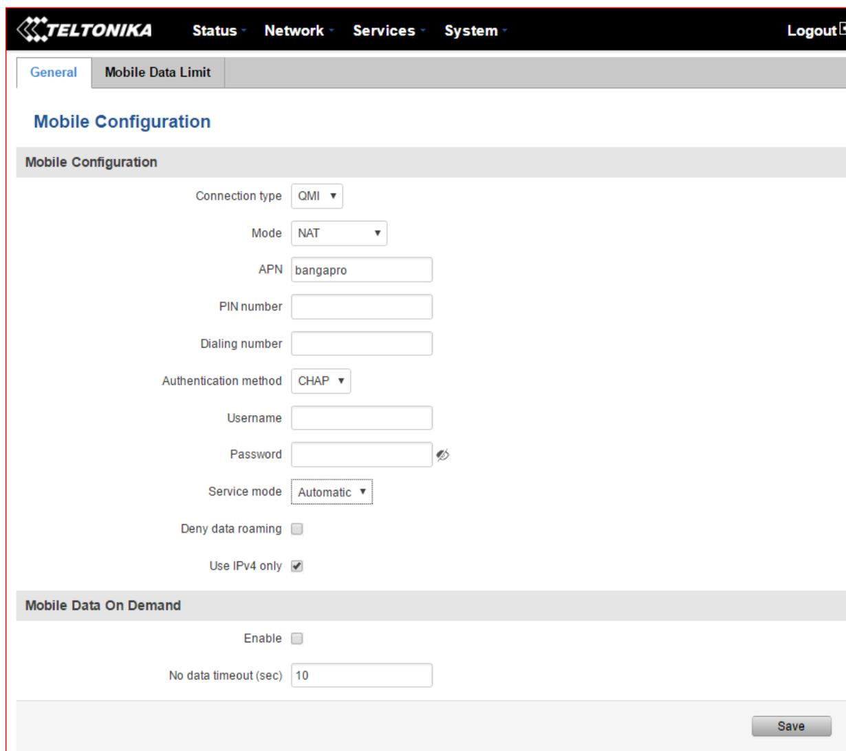
The screenshot displays the Teltonika web management interface. At the top, there is a navigation bar with the Teltonika logo and menu items: Status, Network, Services, and System. A Logout button is located in the top right corner. Below the navigation bar, there are two tabs: 'General' and 'Mobile Data Limit'. The 'Mobile Configuration' section is active, showing various settings for mobile connectivity. The settings include:
