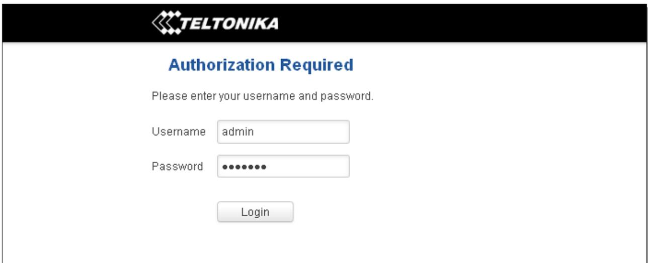
Enter the default password, which is “admin01” into the “Password” field and then either click Login with your mouse or press the Enter key. You have now successfully logged into the RUT240!
