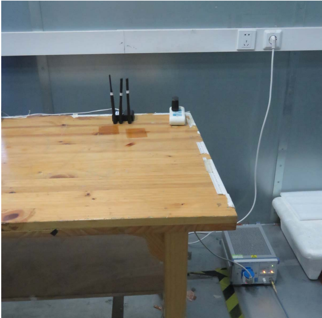
Picture 3 Conducted Emission Test Setup
