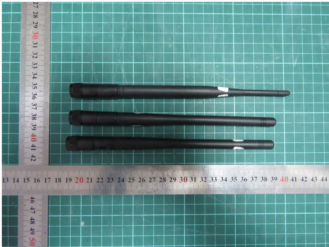
LTE Antenna/ WiFi Antenna
