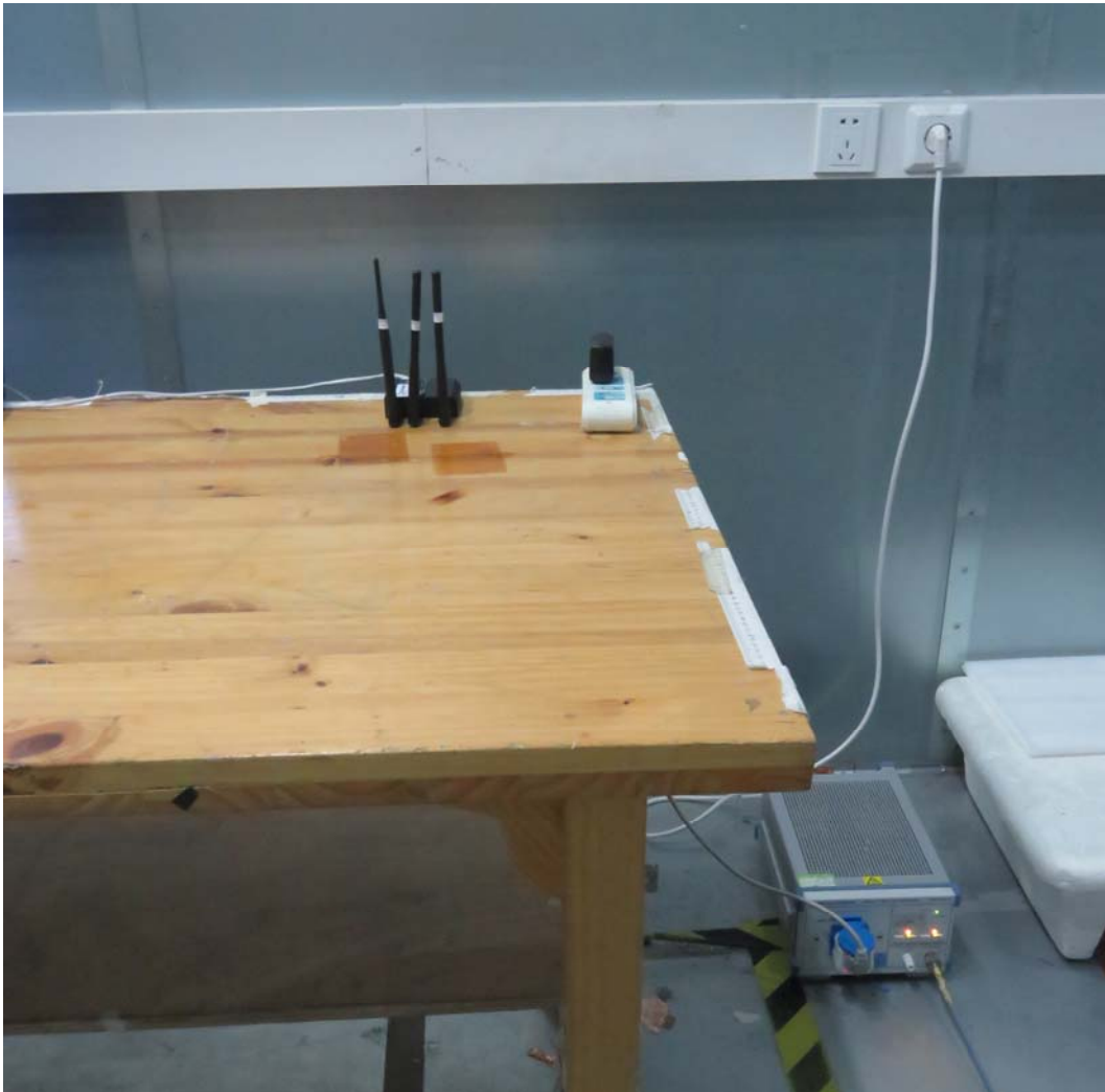
Picture 3 Conducted Emission Test Setup
