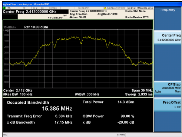
(802.11b) -20dB Bandwidth plot on channel 6
