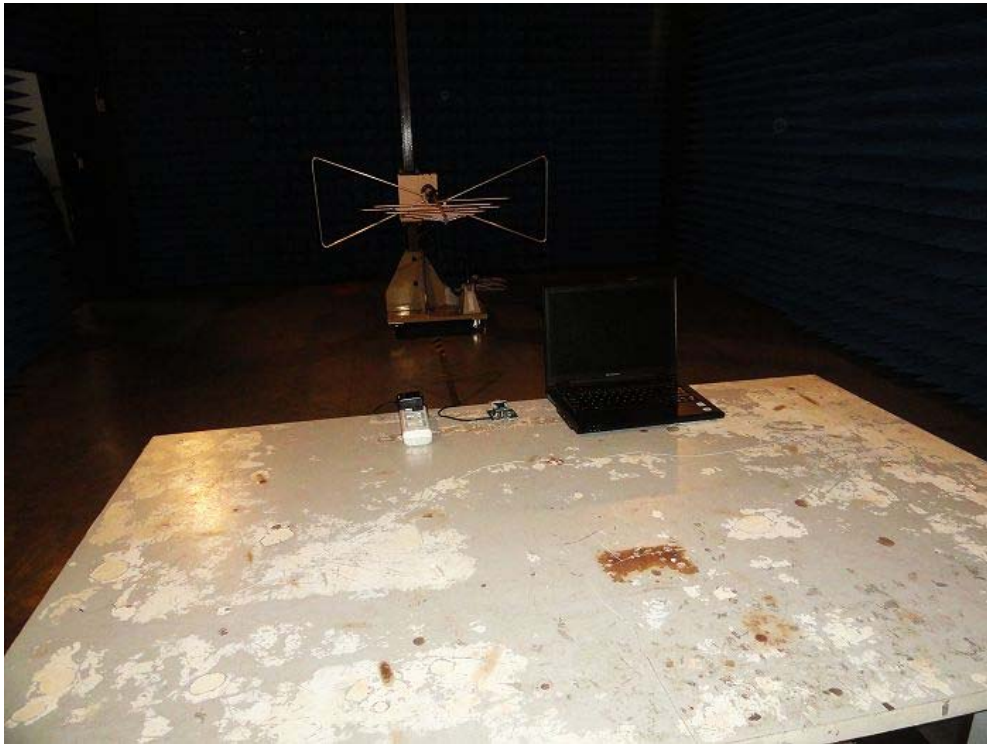
Radiated Emission Test Setup:
