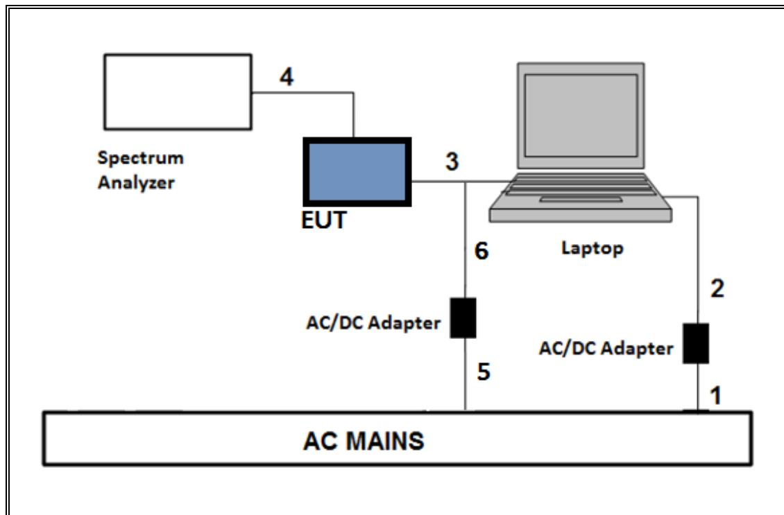
**SETUP DIAGRAM - AC LINE CONDUCTED TEST AND RADIATED TEST**
