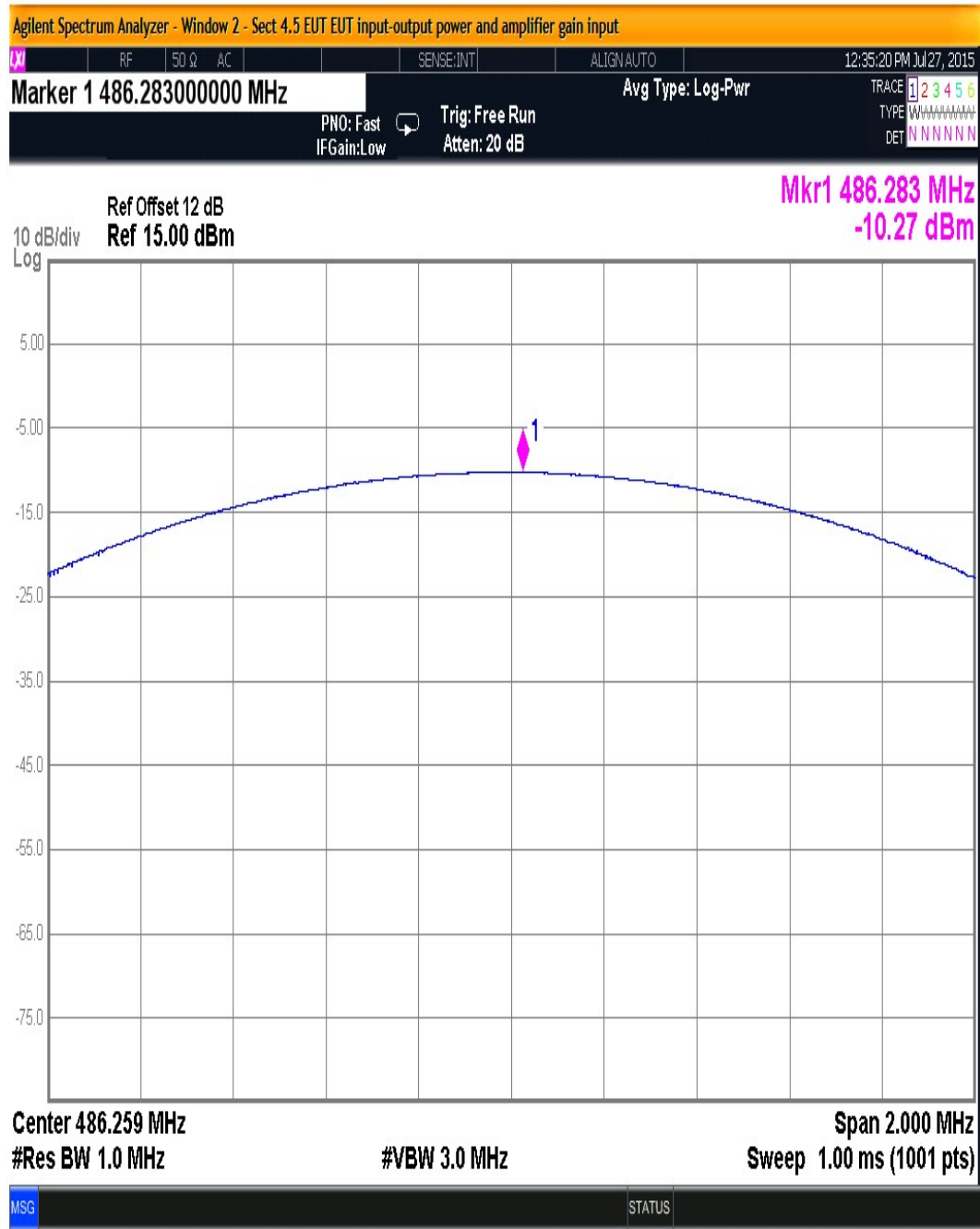
Figure 61. Window 2 - Sect 4.5 EUT EUT input-output power and amplifier gain input
