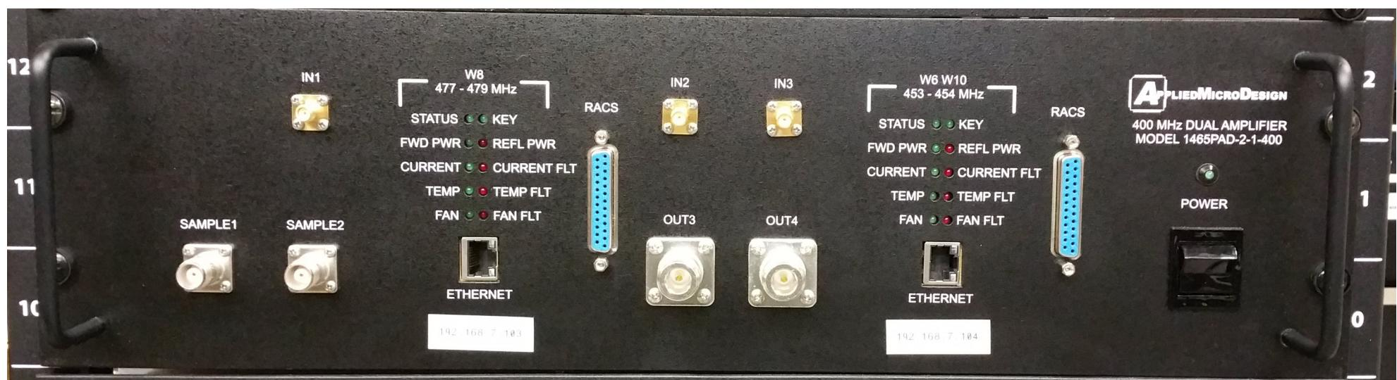
400 MHz Dual Power Amplifier, 3 Input - Front Panel
