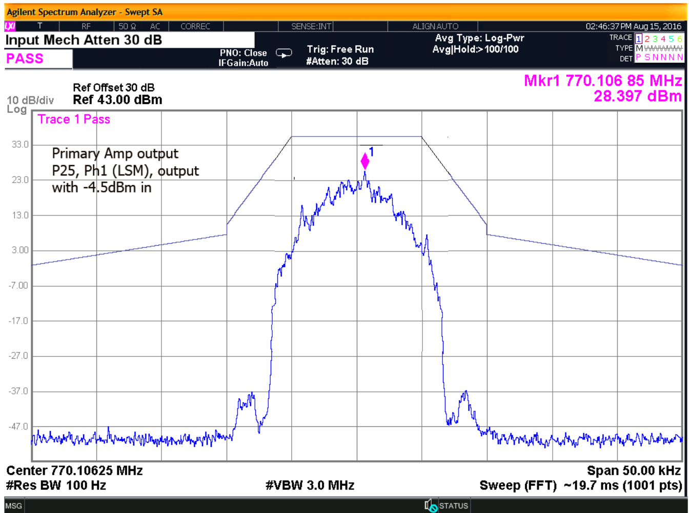
Figure 24: 769-775MHz, P25 Ph1 LSM Output, Mask C- Primary Amp, 0.5dB under AGC
