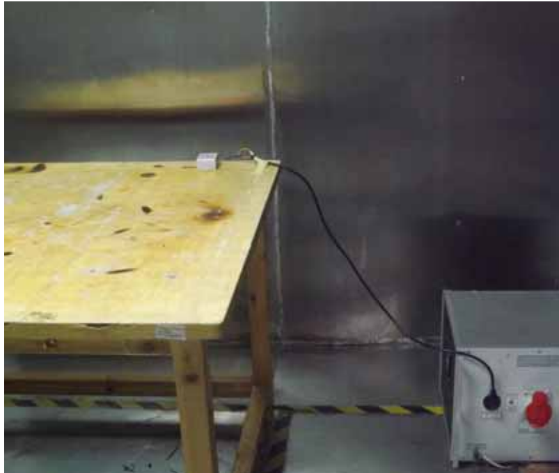
Photograph – Radiated Emission Test Setup for 30MHz ~ 1000MHz at Test Site 2#
