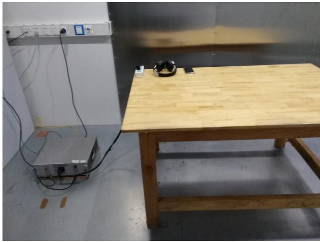
Conducted Emissions Test Setup Front View
