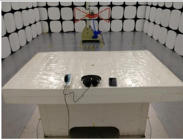
Conducted Emissions Test Setup Front View
