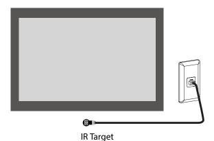
The IR target is used to receive IR signals from a typical remote control. The IR target should be installed in close proximity to the television using the adhesive pad on the rear.
