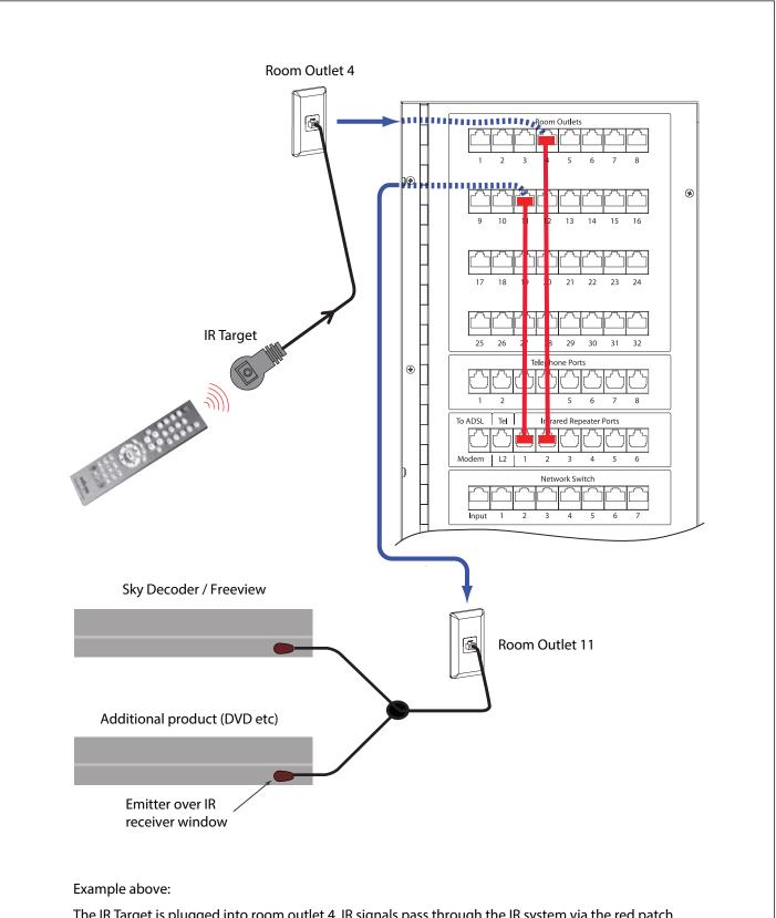
The IR Target is plugged into room outlet 4. IR signals pass through the IR system via the red patch cables, then back out room outlet 11 to control the product.
