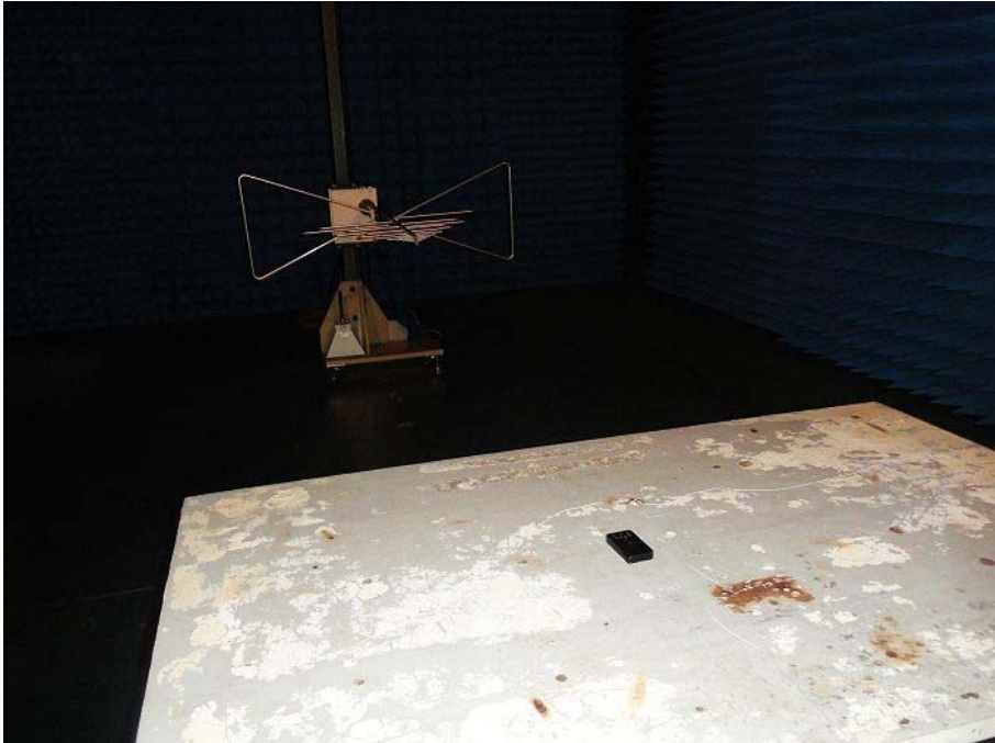
Radiated emission test view
